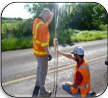
weight is dropped a number of times to achieve a minimum of 25 mm of penetration. The number of blows delivered and the total penetration is entered into the XL template to calculate CBR.
