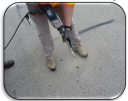
a minimum of 25 mm of penetration. The actual penetration and blows required are recorded. The number of blows delivered and the total penetration is entered into the XL template to calculate CBR.
