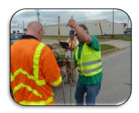
A one-inch diameter hole was bored through the pavement to gain access to the treated base material at several locations. Once the treated material is accessed, the DCP is positioned and the weight is dropped 2 times to seat the cone into the soil. The initial depth is recorded and the weight is dropped a number of times to achieve
