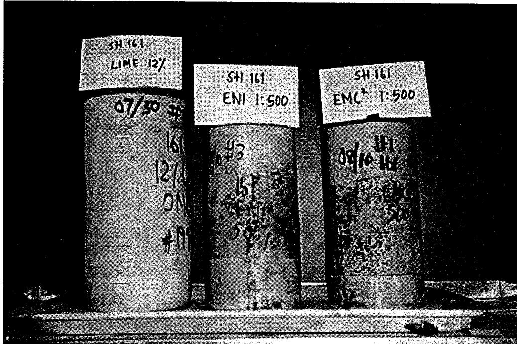
Figure 41. Photographs Showing Comparisons of Swell (Lime -12% Vs EN1-1:500, EMC²-1:500) - SH 161
