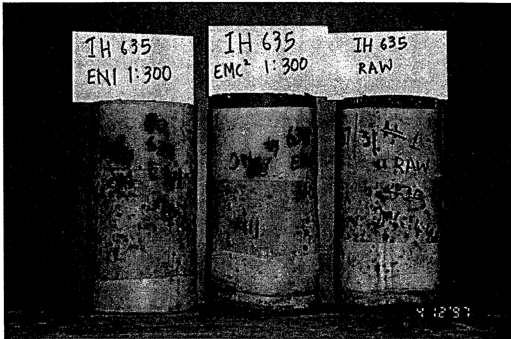
Figure 50. Photographs Showing Comparisons of Swell (Raw Vs EN1-1:300, EMC 2 -1:300) - IH 635
