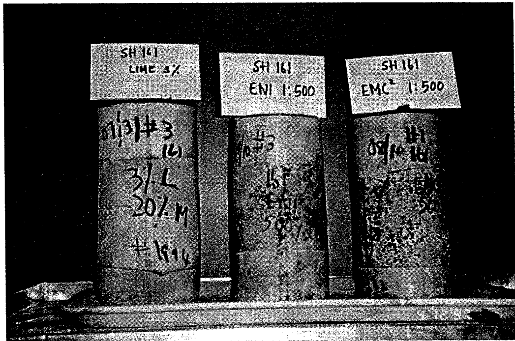
Figure 43. Photographs Showing Comparisons of Swell (Lime -3% Vs EN1-1:500, EMC 2 -1:500) - SH 161
