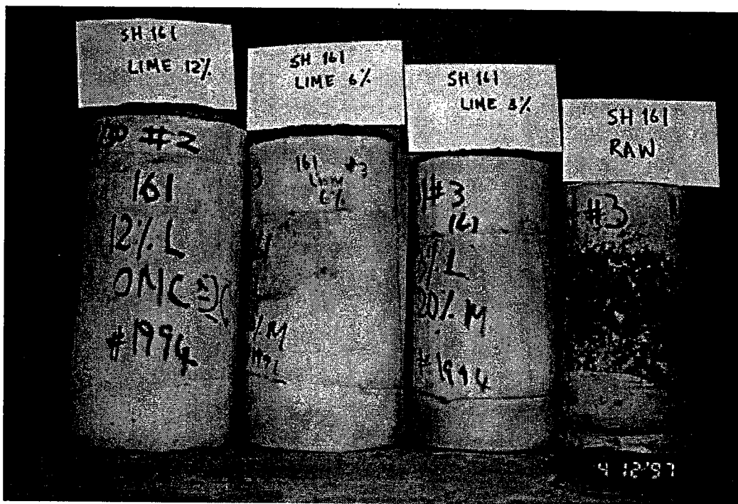
Figure 44. Photographs Showing Comparisons of Swell (Lime with Raw) - SH 161
