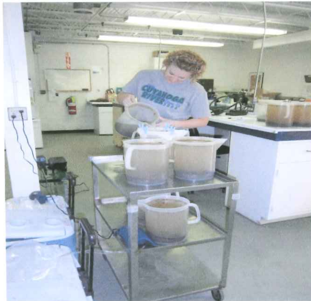
Photograph of Laboratory Preparations for Roadbond EN 1™ Leachate to be Placed in the Tanks
