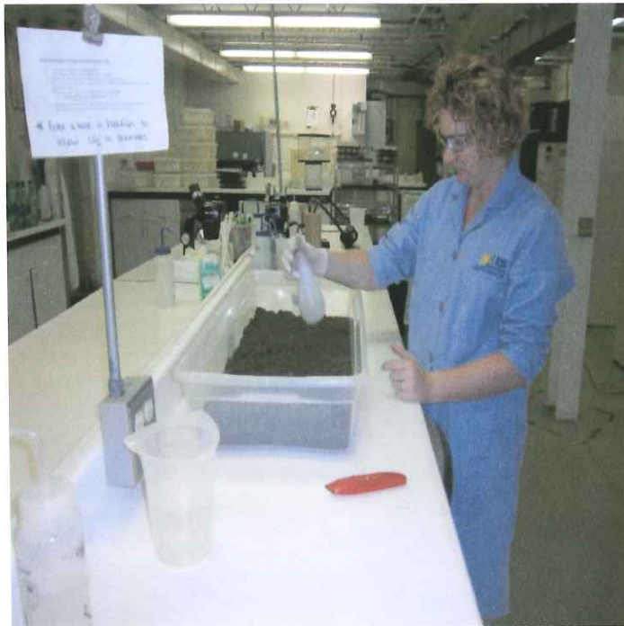
Photograph of Laboratory Soil/Gravel Mix Handling Preparations to Produce Leachate
