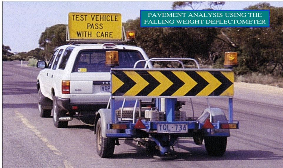
**Figure 9 Dynatest Falling Weight Deflectometer**
